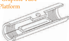
Cross-section of the PerkinElmer HGA graphite tube with manually inserted L'vov platform shown.
