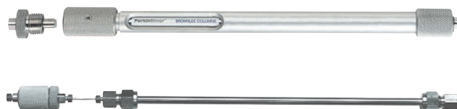
NewGuard cartridges directly coupled to a 220 mm MPLC cartridge and connected externally to a 250 mm conventional column.
