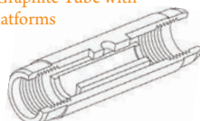
Cross-section of the PerkinElmer HGA graphite tube with integrated platform shown.
