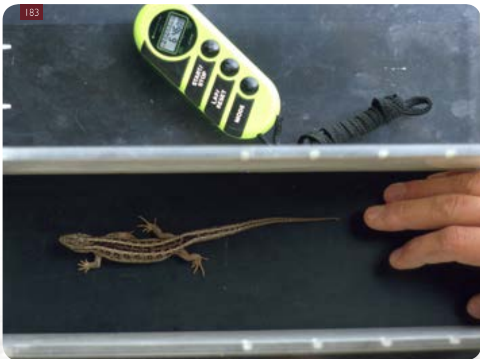
Motorized treadmill used to measure endurance in lizards. The standard speed of the treadmill is 1.0 km/h. The length of time the lizard can run at this speed is taken as the measure of endurance. The lizards are chased to keep them moving
