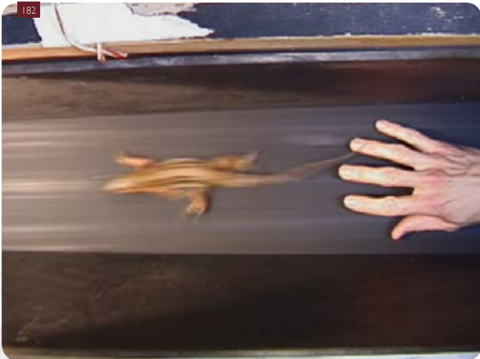
182 High-speed treadmill connected to a computer that can rapidly reach 45 km/h. This is used to measure maximal running speeds of lizards that are chased with the hand simulating a predator
