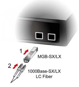
Figure 2-1-7 Plug in the SFP transceiver
