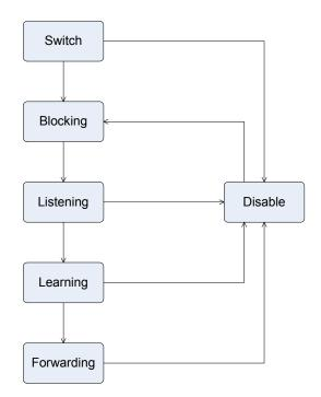
Figure 4-8-1: STP Port State Transitions
