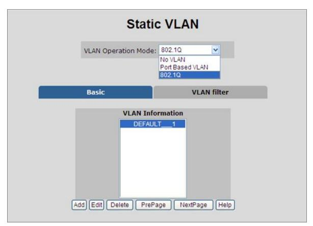
Figure 4-4-2-1: Static VLAN interface
