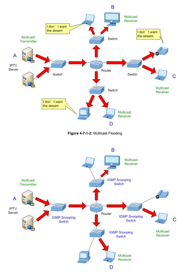
Figure 4-7-1-3: IGMP Snooping Multicast Stream Control
