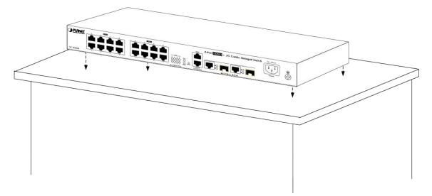
Figure 2-2-1: Place the Managed Switch on the desktop
