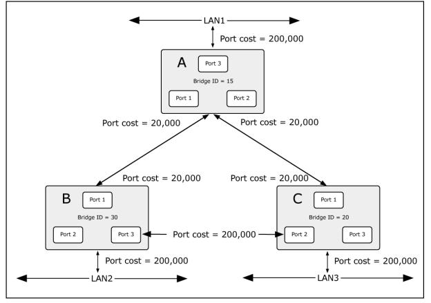
Figure 4-8-2: Before Applying the STA Rules
