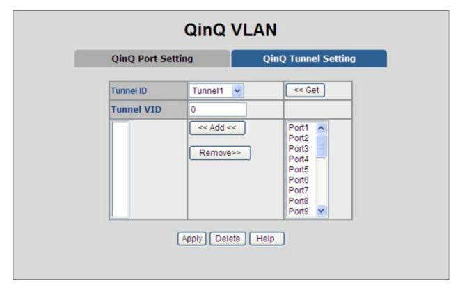
Figure 4-4-5-2: Q-in-Q Tunnel Setting interface
