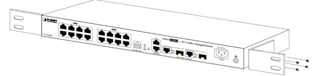
Figure 2-2-2: Attach brackets to VC-820M
