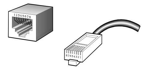
The standard RJ45 receptacle/connector
