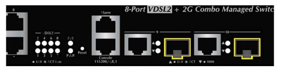
Figure 2-1-5: VC-820M System and Port LED panel
