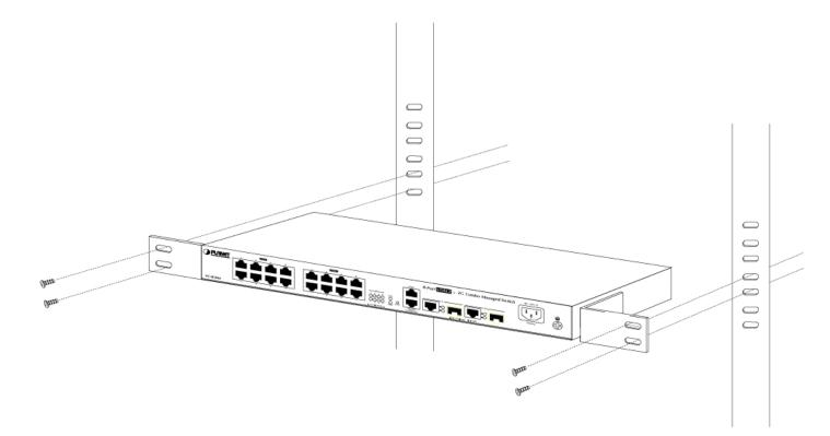
Figure 2-2-4: Mounting the VC-820M in a Rack
