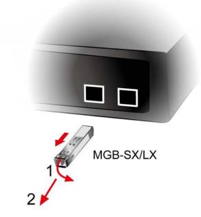
Figure 2-1-8 How to Pull Out the SFP Transceiver
