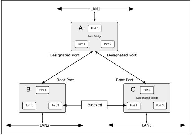
Figure 4-8-3: After Applying the STA Rules
