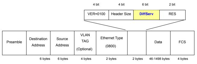
Figure 4-15-4: IPv4 Frame Format
