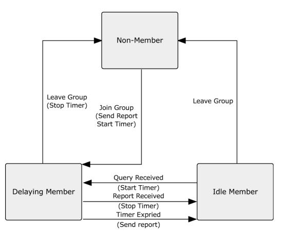
Figure 4-7-1-4: IGMP State Transitions
