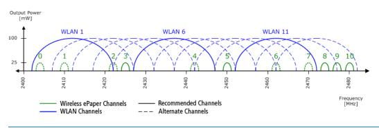
Do not select the same channel for two access points that are in the same area. This causes interference and prevents Displays from joining the network. It is possible to set the same channel on two access points if you are sure that each display is only within range of one of these access points.
