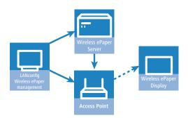
The software consists of LANconfig and the Wireless ePaper Server. LANconfig manages the access points, facilitates their configuration, and invokes the Wireless ePaper management. The Wireless ePaper Server receives the instructions from the Wireless ePaper Management, computes the content to be rendered, and transfers this to the access points. The access points forward the content to the Wireless ePaper Displays by radio.
