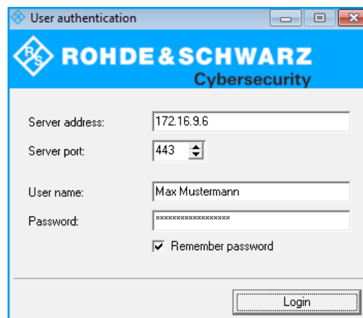
Figure 3-6: User authentication using the R&S Unified Firewalls User Authentication client.
