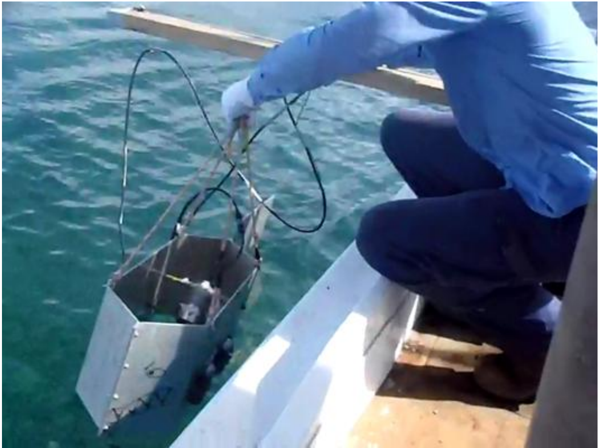
Plate 3-1 Picture showing the video camera being deployed for the benthic habitat video tows
