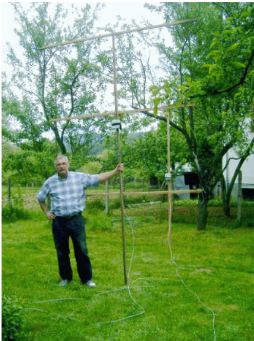
Fig.5 The author at the experimental green field. 4 m 2 4-squares crossed parallel loop is mounted on a wooden frame..
