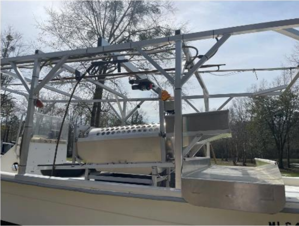
Figure 7. Photograph of a Tumbler/Sorter/Washer (Top); Photograph of a Refrigeration Unit Installed in Bed of Pickup Truck (Bottom).
