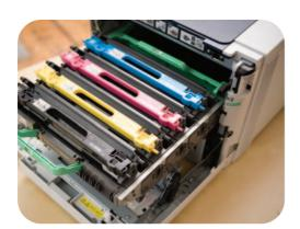
Brother's innovative arrangement of toners and drums can be accessed from the front of the machine. This allows fast, efficient and easy toner and drum replacement.
