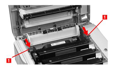
**3.** Hold the fuser **by its handle**. Lift the fuser out of the printer. If the fuser is still warm, place it on a flat surface which will not be damaged by heat. After letting the fuser cool down, discard it.
