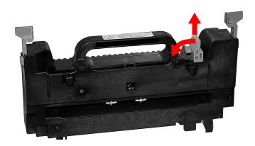
**6.** Hold the new fuser by the handle. The fuser pressure release lever (1) should be on the right. Lower the fuser into the printer.
