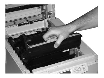
**9.** Remove the orange drum seal.
