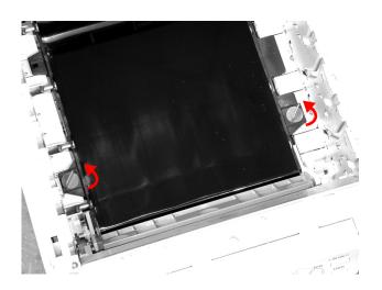
**6.** Pull up the handle and lift the belt unit out of the printer.
