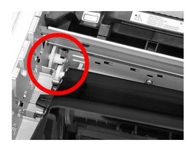
**9.** Turn the two belt locks about 45° clockwise to secure the belt unit in place.
