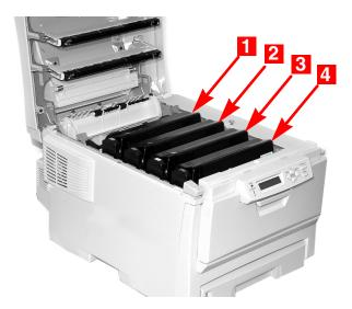
**3.** Pull the colored toner release lever on the cartridge to be replaced towards the front of the printer. Shown: replacement of the black toner cartridge
