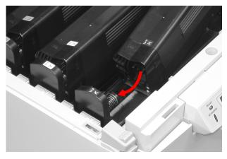
**8.** Lower the right end of the cartridge into the image drum unit. Press it firmly down in place. Then, push the colored lock lever back to open the toner slot and lock it in place.
