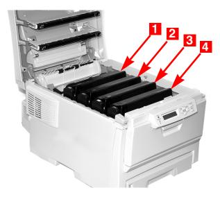
**3.** Lift each of the image drum units out of the printer. Place them on a *flat* surface in a safe place away from direct sources of heat and light.
