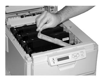
**10.** Install the new toner cartridge in the image drum. See "Install a Toner Cartridge" on page 57.
