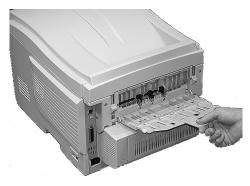
Open the face up stacker at the rear of the printer and pull out the tray extension.
