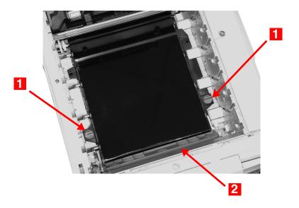
**5.** Turn the two locks about 45° *counterc*lockwise to release the belt.
