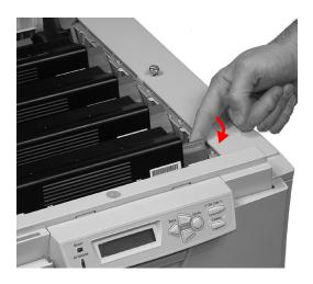
**4.** Lift the right-hand end of the cartridge. Then, pull the cartridge to the right to release the left-hand end. Remove the toner cartridge. Discard it in accordance with your local regulations.
