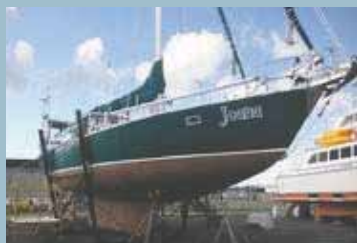
Coppercoat applied 2008, now 10 years old
