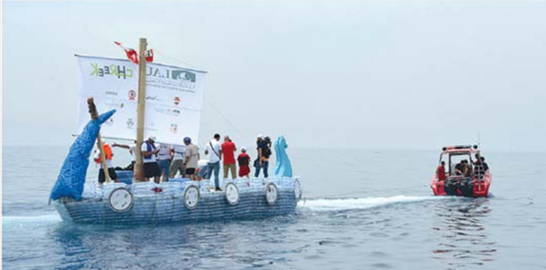
In an effort to revive Lebanon's heritage through saving its environment, a team of SOE students partnered with the Lebanese environmental NGO Chreek to build a replica of a Phoenician trireme. The replica trade ship was constructed out of 100,000 up-cycled water bottles and successfully sailed down the coastline from Byblos to Beirut's Zaitounay Bay.
