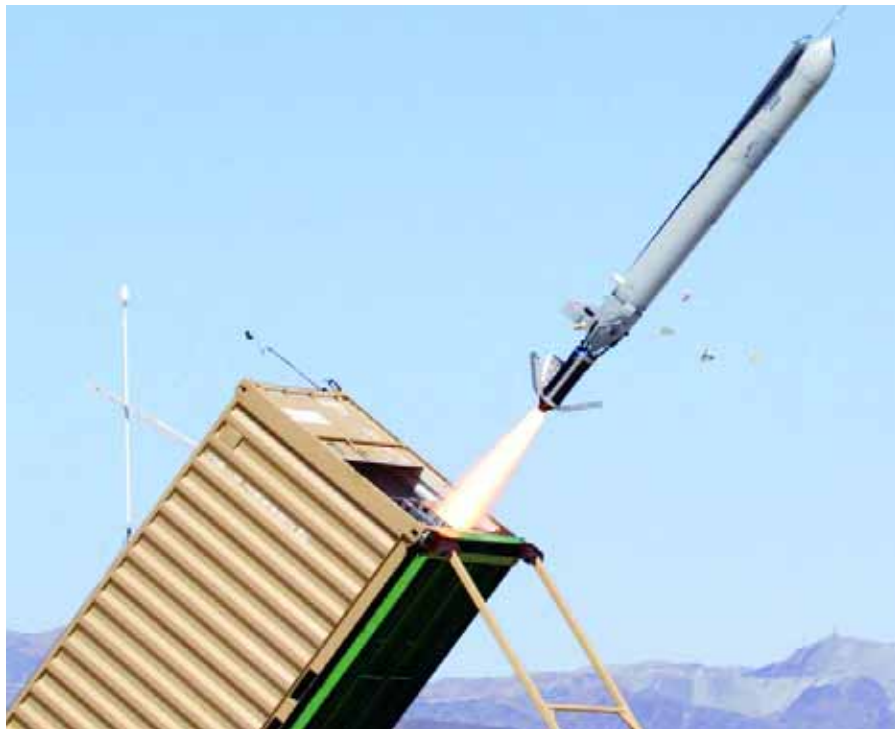
Launched by a small rocket booster and powered in flight by a small turbojet engine, Titan's Affordable Weapon can fly to a target area and loiter for several hours until directed to a specific objective by a forward observer.
