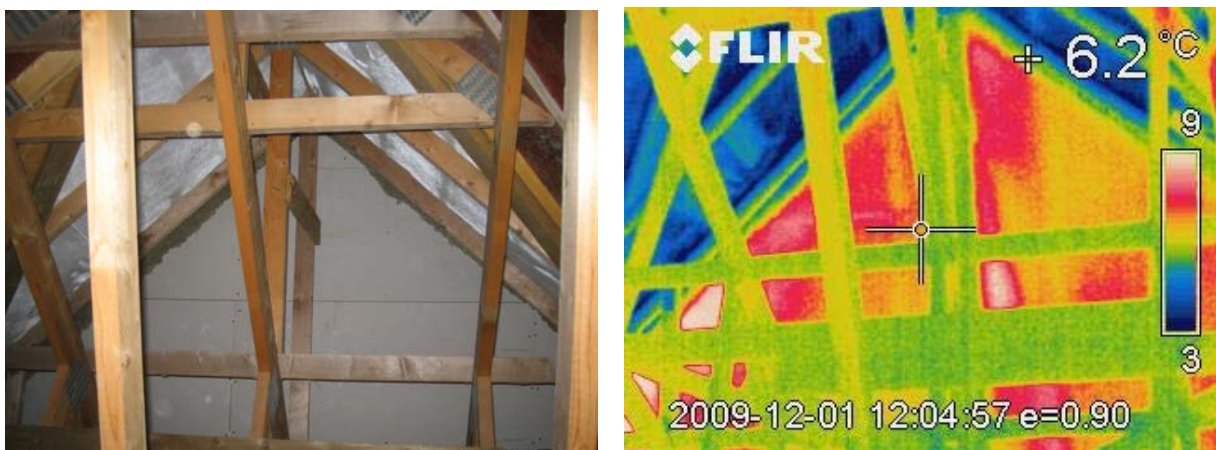
Figure 28 – Photograph and Thermal Image of Party Wall in Loft of House No.15
