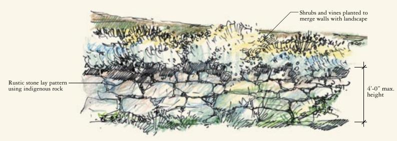
FIGURE 2.1: Retaining wall design
