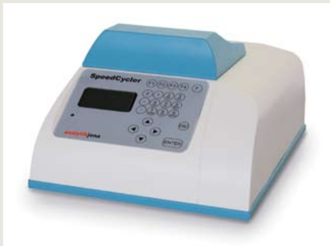
Figure 4 Rapid heat block thermocycler (SpeedCycler, Analytik Jena) and ultra-thin walled microwell plate.
