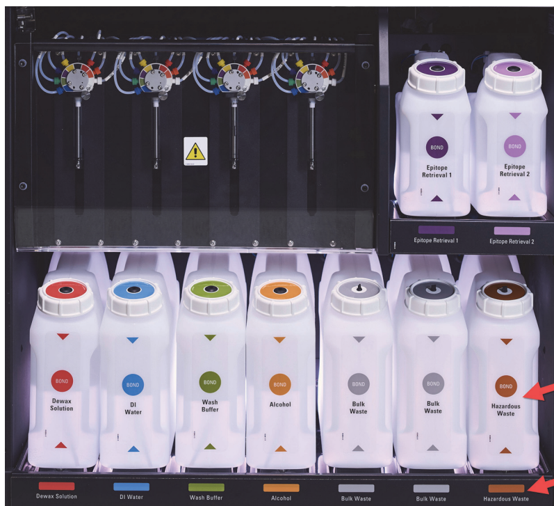
Figur 15: BOND-III bulkreagensbeholdere i position
