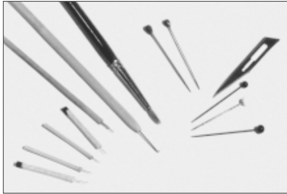
Figure 8-4. Spreading tools (clockwise from lower right): Short- and long-handled setting needles; L-shaped tool; camel hair brush; wax-headed sewing needles; #11 surgical blade; glass-headed pins.
