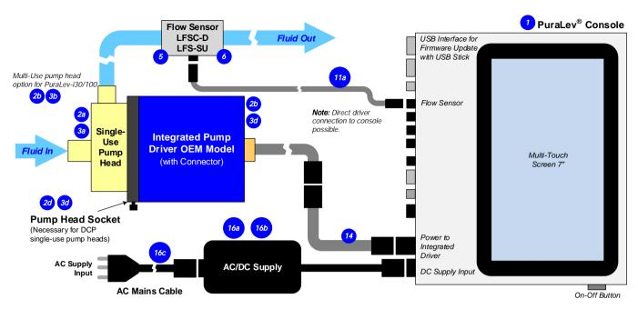
Figure 8: Stand-alone pump system configuration of LCO-i100 console and PuraLev® i30/100 pump systems with flow control or flow monitoring
