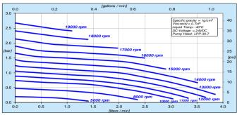
Figure 4: Pressure/flow curves with PuraLev® i30MU (LPP-30.7 pump head)
