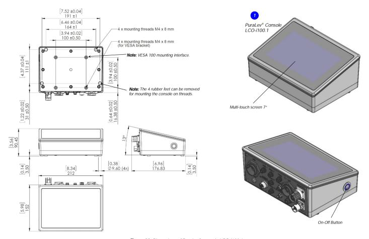
Figure 11: Dimensions of PuraLev® console LCO-i100.1 Note 1: Dimensions in mm and [inch]. Un-tolerated dimensions are for reference only.
