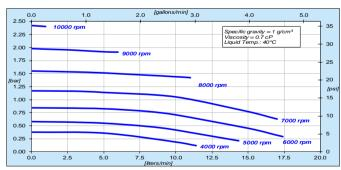
Figure 6: Pressure/flow curves with PuraLev® i100MU (LPP-200.16/17 pump heads)
