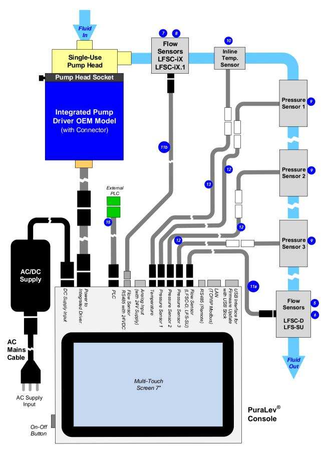
Figure 10: Extended monitoring configuration of console LCO-i100 for advanced fluid handling in bioprocessing applications
