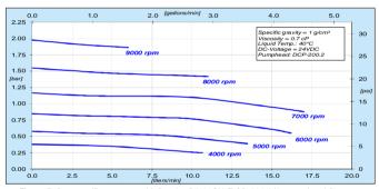
Figure 5: Pressure/flow curves with PuraLev® i100SU (DCP-200.2/3 pump heads)
