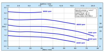
Figure 7: Pressure/flow curves with PuraLev® i600SU (DCP-600.2 pump head)
