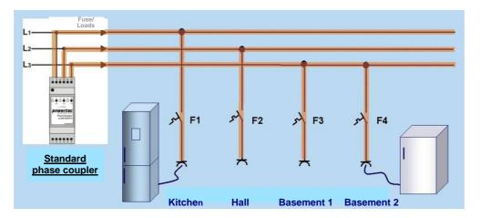
The phase coupler permits data transmission from one phase to the other phases, enabling the appliances to communicate.
