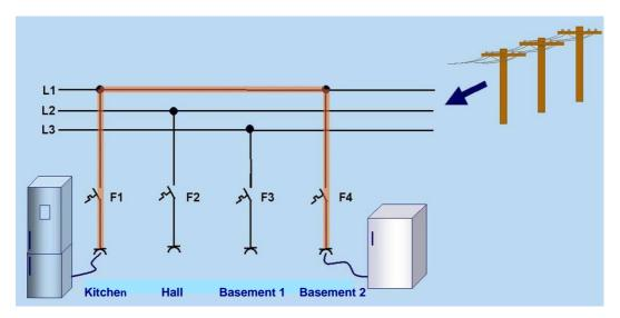
If the setup cannot be carried out successfully once the appliances have been installed, then they are presumably not connected to the same phase. In that case an electrician has to install a so-called phase coupler in the fuse box.
