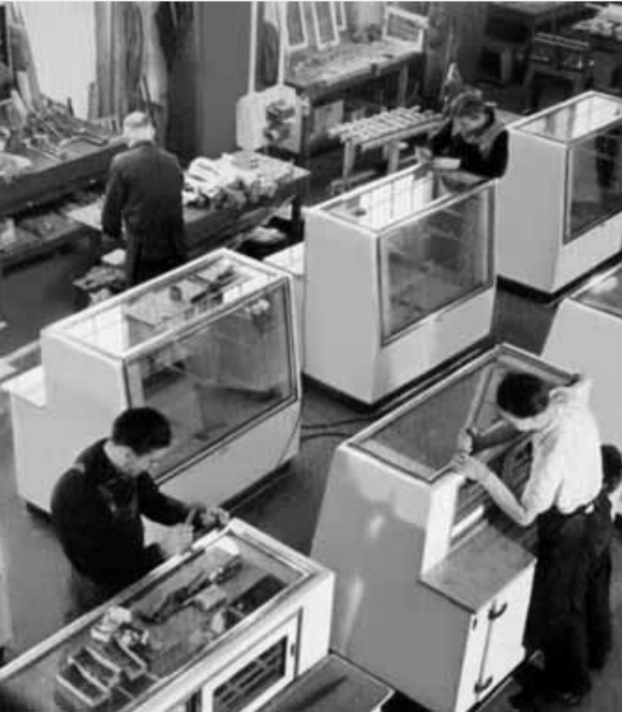
Building refrigerated display cases in the factory in Mainz-Kostheim (approx. 1950).
