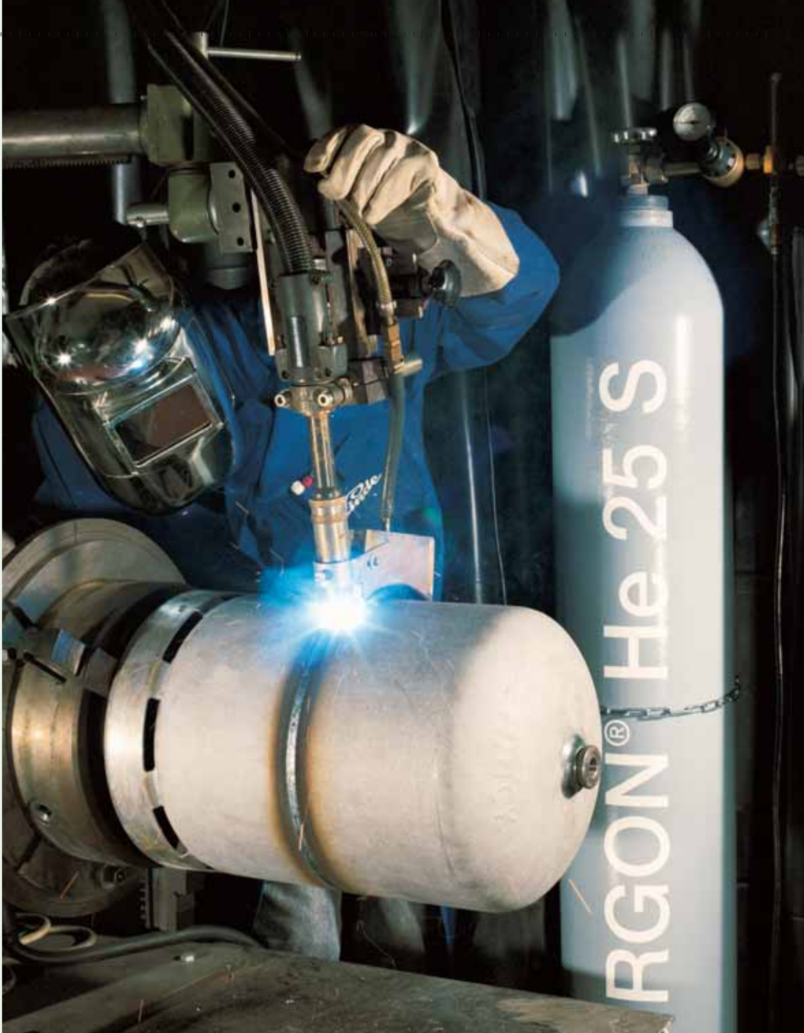
Welding with the protective gas "Corgon" from Linde.
