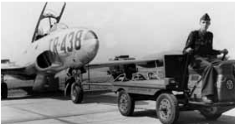
A Güldner Hydrocar tows an air force plane. These vehicles were built from 1958 to 1965 in Aschaffenburg.
