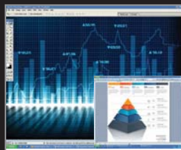
PIP View: A source video can be displayed as a free floating image over the main video signal
