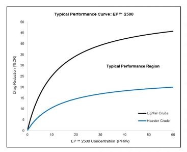
This performance curve demonstrates the range in which EP<sup>™</sup> 2500 Flow Improver can operate, depending on pipeline and fluid conditions.
