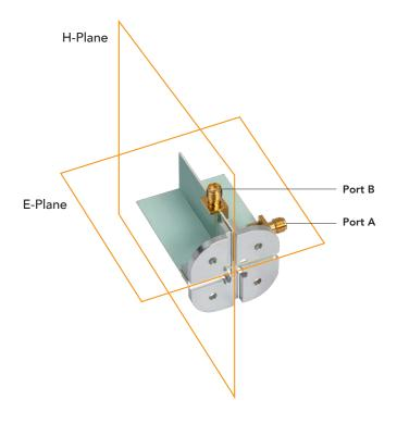
Illustrated below are the plane of electric field (E-plane) and magnetic field (H-plane) vectors observed with respect to the direction of maximum radiation from Port B.
