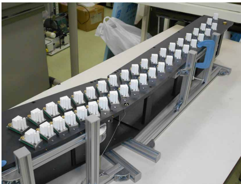
Fig.3. Photograph of the detector case of the tagger with all the counter units mounted on it.
