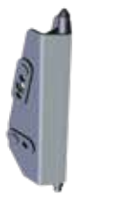
C-152 | C-15 UNIVERSAL CONVERSION KIT Convert other brand loaders to Snap-Attach. Kit contains: Two C-15 universal couplers with 1" pins and two female adapters for attachment. Optional bushing kits adapt unit to various pin diameters. Note: Loader arm ends must be 4.5" or less and cylinders located on the top of the loader arms.
