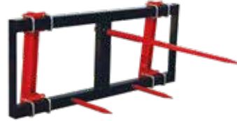
SP-43 | SP-76 THREE-PRONG BALE SPEARS The SP-43 is for the 20 and 40 series loaders. Use the SP-76 with wider framed 70 series loaders. Quality heat treated forged steel spears ensure easy penetration and release. Both units include one long spear and with two short stabilizing spears. (Long spear is 49-1/4" long with 44" usable length)
