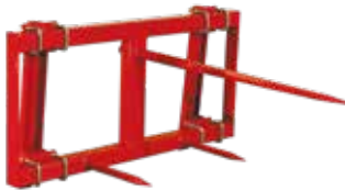
SP-43 | SP-76 THREE-PRONG BALE SPEARS The SP-43 is for the 20 and 40 series loaders. Use the SP-76 with wider framed 70 series loaders. Quality heat treated forged steel spears ensure easy penetration and release. Both units include one long spear and with two short stabilizing spears. (Long spear is 49-1/4" long with 44" usable length)
