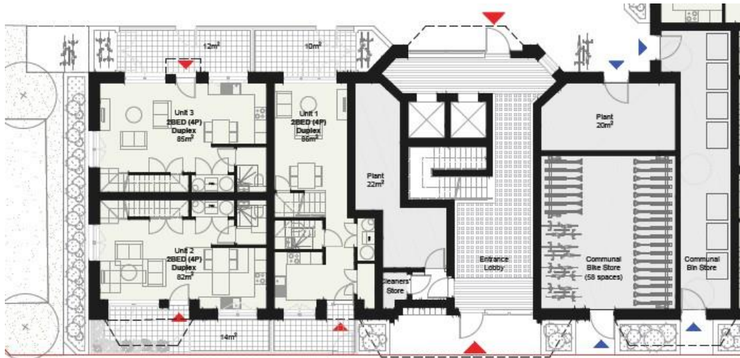
Figure 17: Ground floor extract detailing residential entrance off Vauxhall Street, bike store and three ground floor maisonettes
