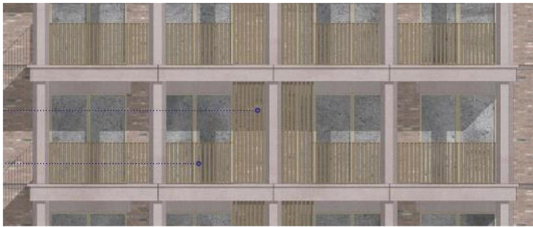
Figure 48: Image of Jonathan Street building south elevations showing angles privacy screens and balustrades (source: Design and Access Statement)
