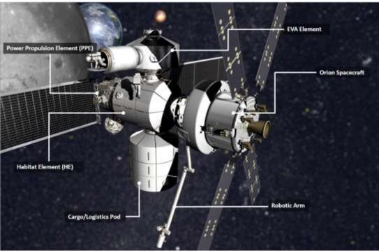
Figure 1. Lockheed Martin's Phase 1 DSG in Cislunar Space
