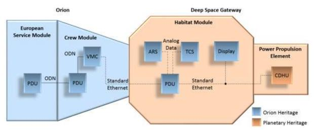
Figure 5. Significant Components in DSG Network Architecture
