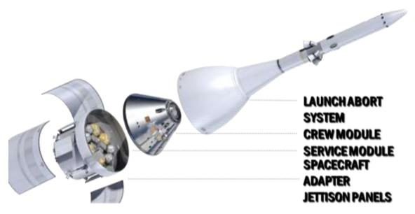
Figure 2. The Orion Spacecraft Configuration
