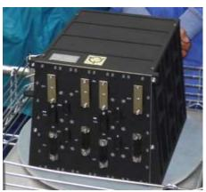
Figure 4. Orion Vehicle Management Computer houses the Flight Control Modules that are the command source for the spacecraft and could minimize computing needed on the DSG.
