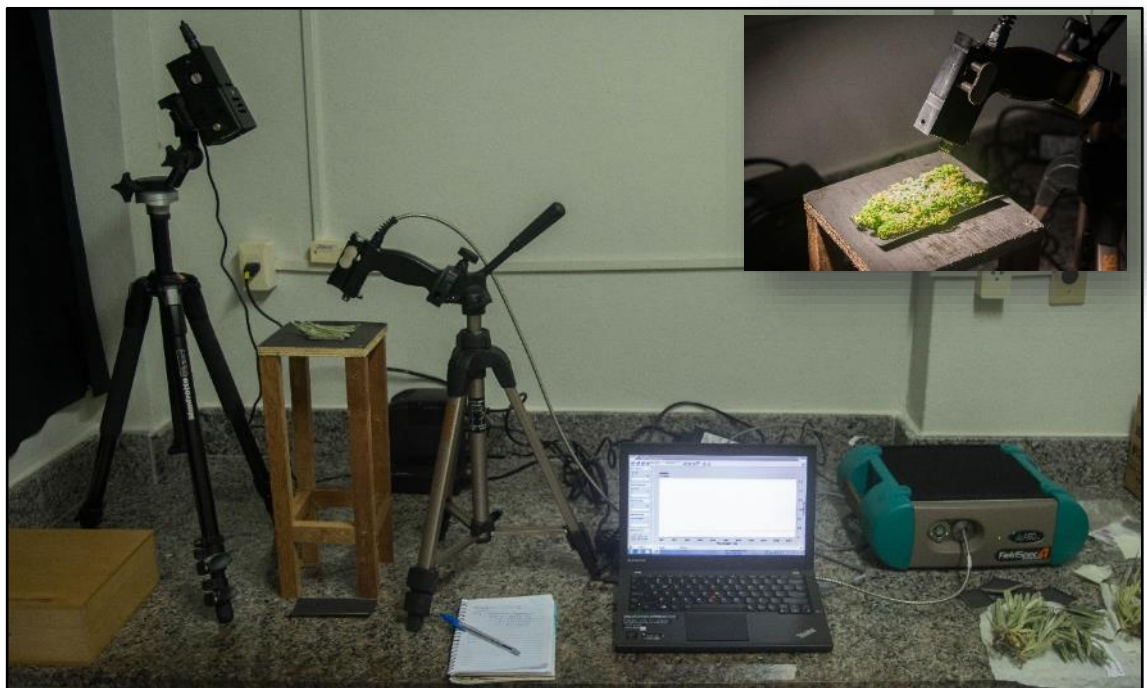
Figure 2 - ASD Spectrophotometer with the spectral probe. A detail of the material at the moment of spectra capture.
