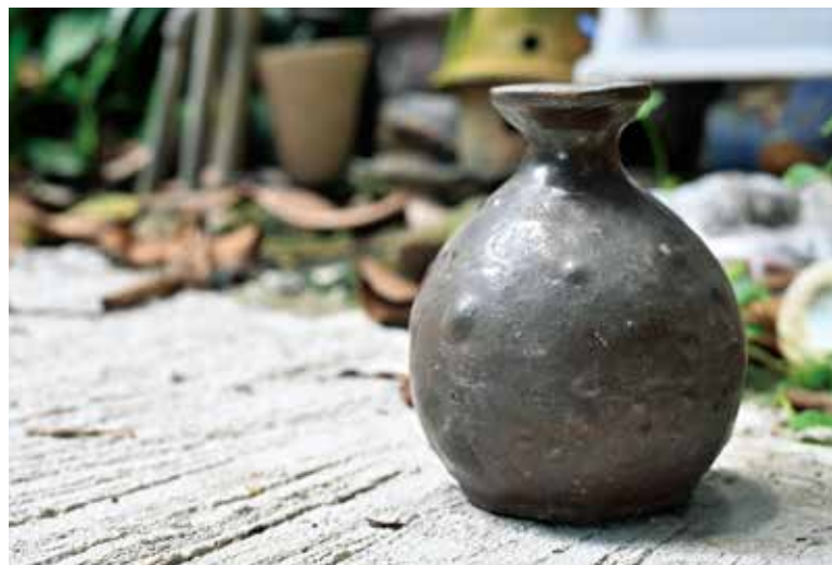
不能出售的次貨——表面滿布氣泡的陶酒樽。 Not good enough to sell — a wine bottle pockmarked by air bubbles in the clay.
