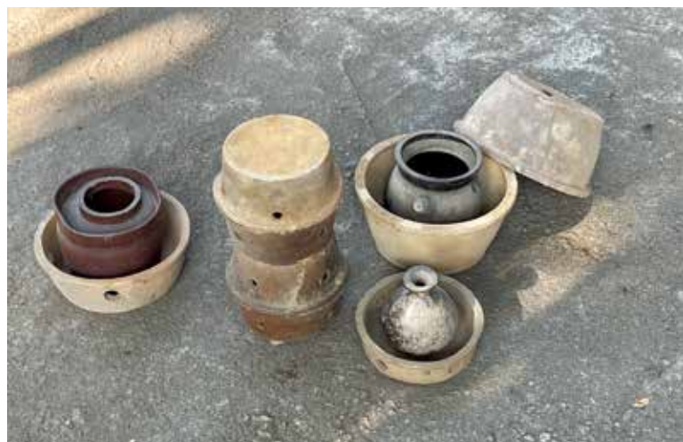
右 工合陶窯備有大小不同的匣钵。 L Saggars protected the products during firing, and could be stacked to make maximum use of kiln space. R Kung Hop's saggars came in several sizes.
