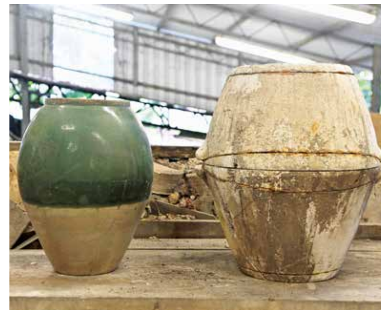
金塔模具分為兩部分，合共高 62.5 釐米，最寬處的内圈直徑為 48 釐米。 The 2-part plaster mould for the reburial urn is a whopping 62.5 cm tall and 48 cm in diameter.
