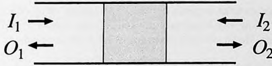
Figure 1.3: Schematic representation of the transport through the conductor. Incoming states ( I ) are scattered into outgoing states ( O ).
