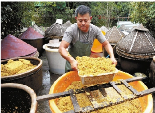
Factories stock flowers by salt water(water:salt :alum=100: 30: 3) which will not deteriorate for about one year .
