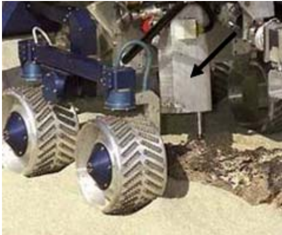
Figure 1. An engineering model of Mini-Corer was installed on JPL's field test rover, FIDO, to facilitate basic mission operations testing (see arrow). The Mini-Corer mass is 2.7 kg and the Mini-Corer box dimensions are 29.8 cm x 14.51 cm x 9.64 cm. This model currently resides at JPL.[2]
