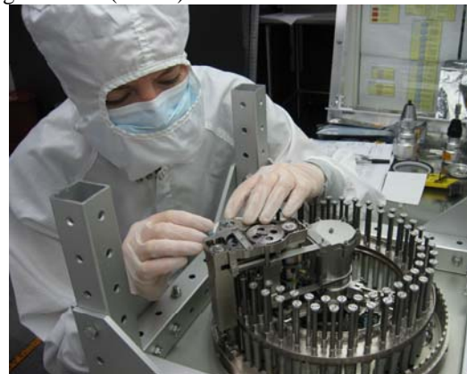
Figure 6. The Sample Manipulation System was developed for Mars Science Laboratory Sample Analysis at Mars instrument. It has 74 cups that transfer a sample to a pyrolysis oven and make a hermetic seal with the oven.
