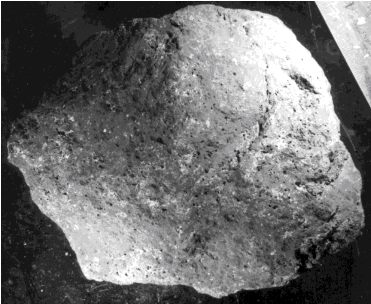
Figure 2: Original photo of rounded, dust-covered, surface of 10017,0. NASA S69-47573. Note micrometeorite craters and vesicles. This was originally thought to be the “top” surface until ^{56}\text{Co} was found on the other side (figure 3).
