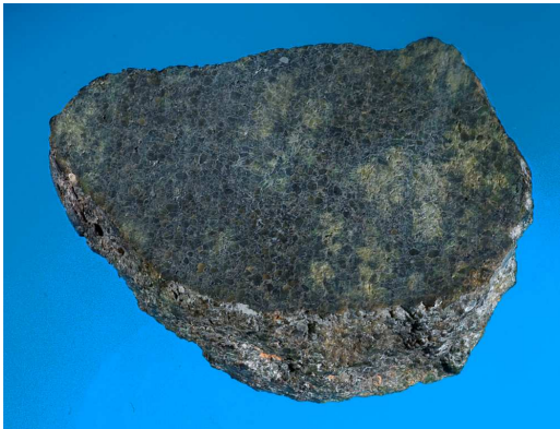
Figure 1. Cut Northwest Africa 6342 stone (width 4 cm) showing regions rich in olivine (yellow-green) and pyroxene (dark gray).
