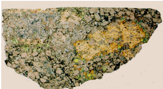
Figure 2. Partially cross-polarized light thin section image showing different textural domains. Dark regions are feldspathic melt pockets. Width = 23 mm.
