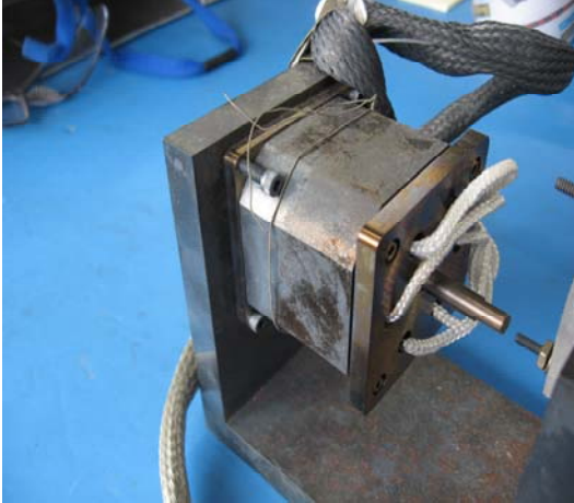
Figure 4.59: High-temperature DC motor (Honeybee).
