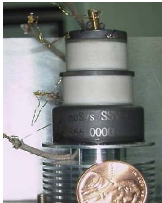
Figure 5.10: High temperature vacuum triode including heater, cathode, grid, and anode.
