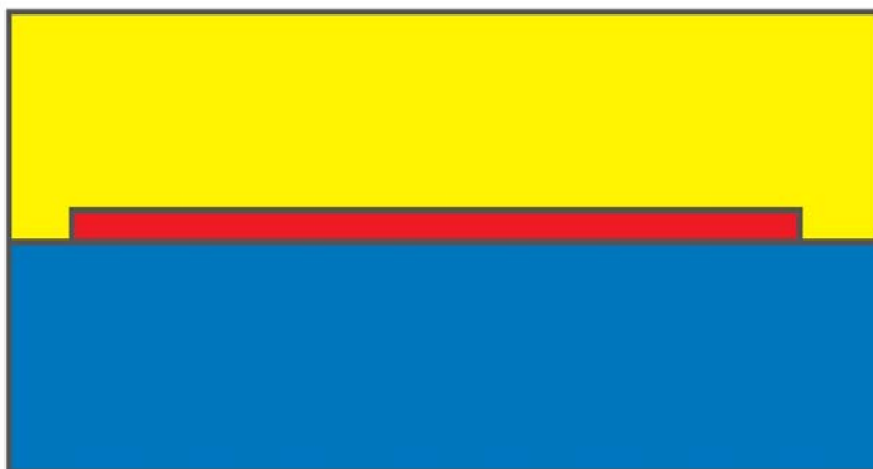
Figure 4.19: Cross section of the flux plate. The yellow material is a 1-cm thick low conductivity material, the red slab is a 1-mm thick copper plate, and the blue is high conductivity, conformable material with a thickness of 1 - 2 cm.
