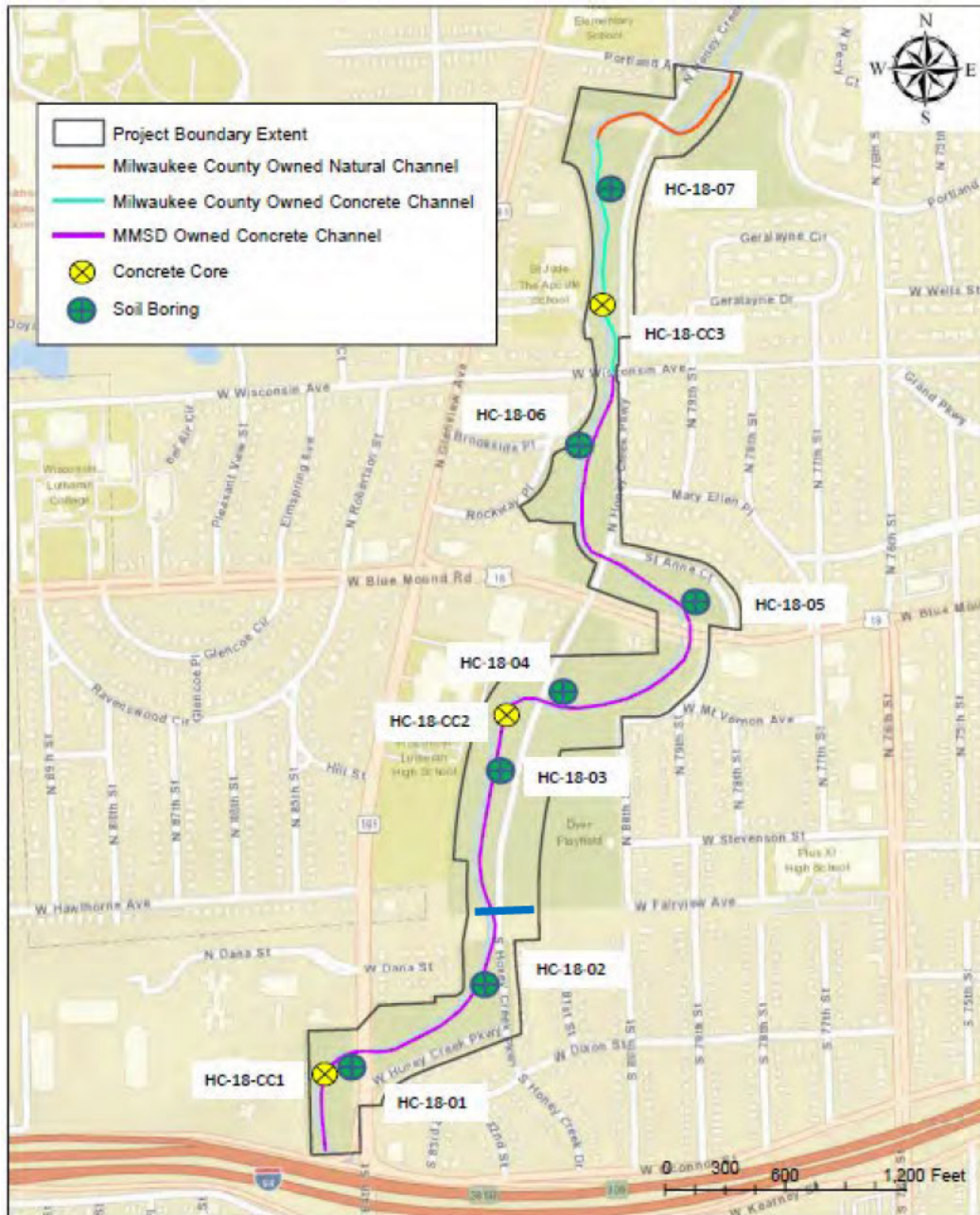
Figure 27: Phase 2 ESA sampling map. Blue line indicates new upstream (southern) project limit.
