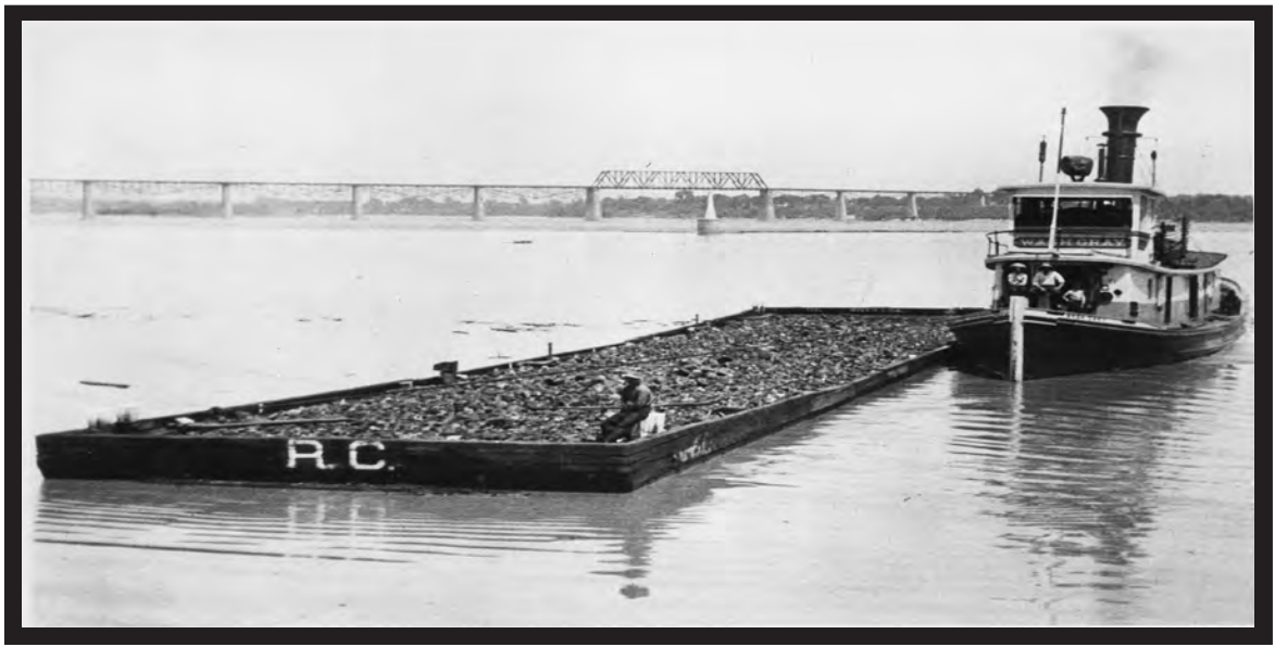
Falls piloting near the turn of the century involved using harbor towboats, such as the Wash Gray, to shuttle coal barges owned by the River Combine through the canal or over the Falls. The dam built at the turn of the century is visible in the background upstream of the Ohio Falls bridge. (Murphy Library, University of Wisconsin)
