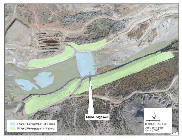
Figure 3: Revegetation design for the Calico Ridge Weir.
