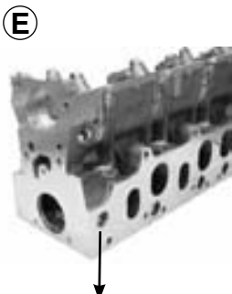
E Thermo-contact M 14 x 1,25 Thermo-contact M 14 x 1,25 Thermocontact M 14 x 1,25 Thermoschalter M 14 x 1,25
