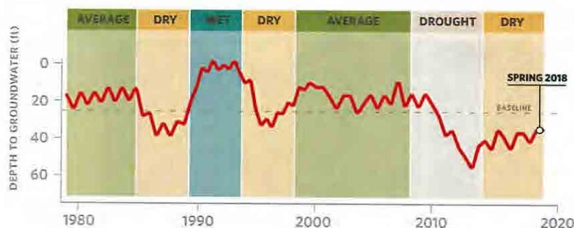
Figure 3. Example seasonality and interannual variability in depth to groundwater over time. Selecting one point in time, such as Spring 2018, to characterize groundwater conditions in GDEs fails to capture what groundwater conditions are necessary to maintain the ecosystem status into the future so adverse impacts are avoided.
