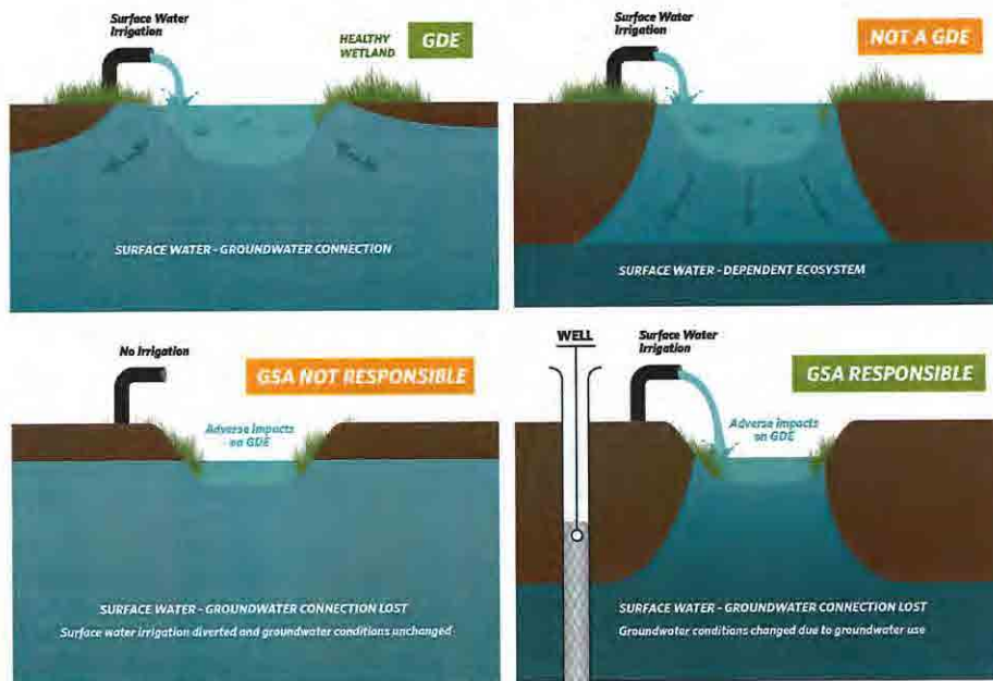
Figure 4. Ecosystems often depend on multiple sources of water. Top: (Left) Surface water and groundwater are interconnected, meaning that the GDE is supported by both groundwater and surface water. (Right) Ecosystems that are only reliant on non-groundwater sources are not groundwater-dependent. Bottom: (Left) An ecosystem that was once dependent on an interconnected surface water system, but loses access to groundwater solely due to surface water diversions may not be the GSA's responsibility. (Right) Groundwater dependent ecosystems once dependent on an interconnected surface water system, but loses that access due to groundwater pumping is the GSA's responsibility.
