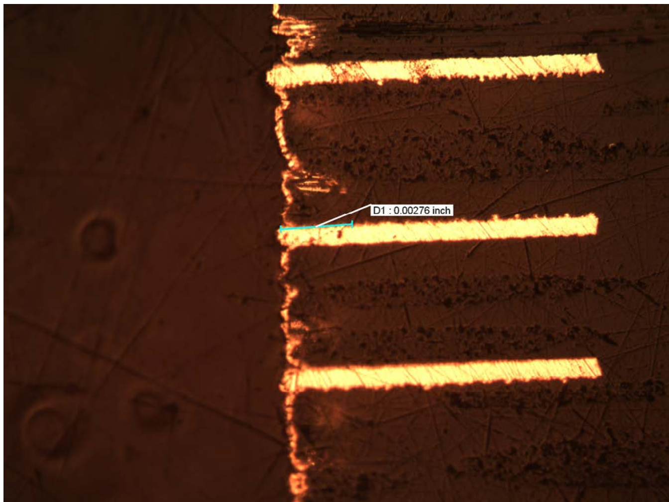
Figure 2: Wicking in test boards with this particular polyimide following etchback and electroless copper deposit could not meet the IPC Class 3A limit despite strict adherence to the recommendations from the material supplier and several process adjustments.
