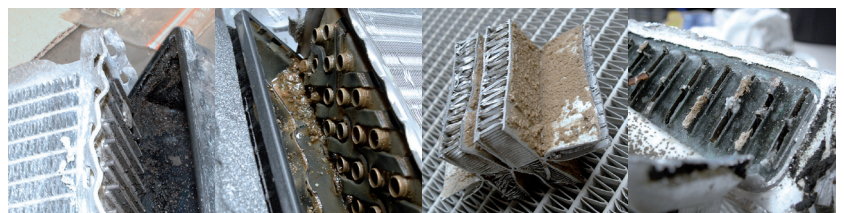
Figure 2: Deposits like rust, limescale, sealant, or other foreign objects cause blockages and reduce cooling performance.
