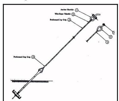
Figure B-7: Installed Ground Anchor
