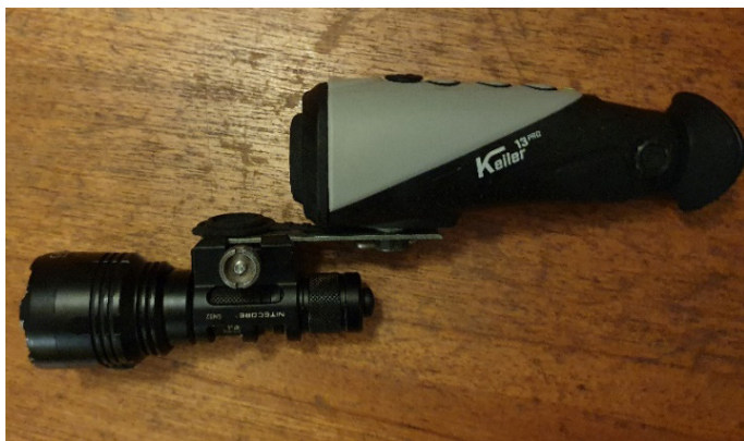
Construction of torch attached to thermal scope helps to find rodents.
