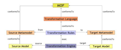
Figure 3.4: Basic Concepts of Model Transformation
