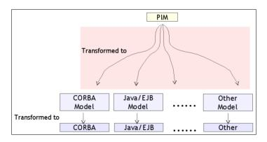
Figure 3.3: MDA based development Process
