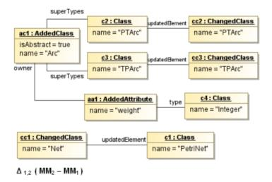
Figure 6.7: Subsequent Petri Net metamodel adaptations
