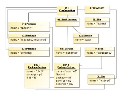
Figure 5.3: Sample Configuration model
