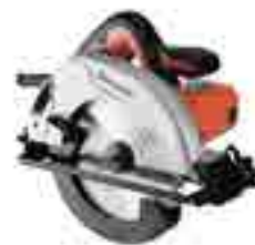
CIRCULAR SAW T-582 Rated input Power: 1050W Blade diameter: 190mm(7-1/2") No-load speed: 4900r/min Rated Voltage: 220V~
