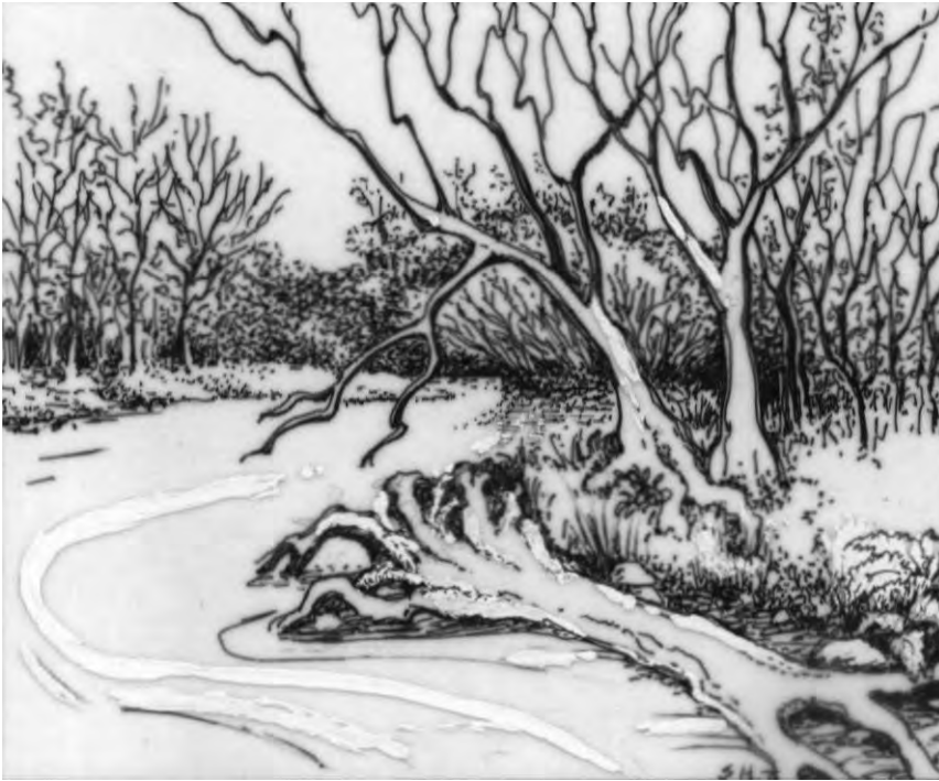
Woody debris repositioned to create habitat while reducing streambank erosion and sedimentation problems.
