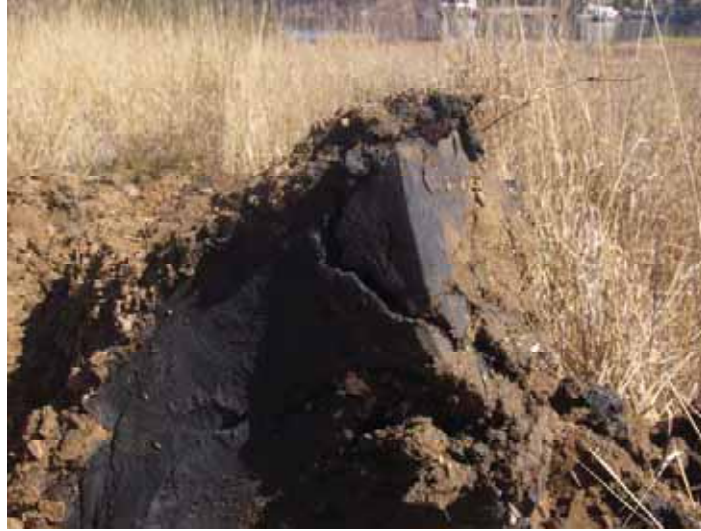
Photo 4. Deep, bay clay extracted from Trench 1. Note retention of bucket shape
