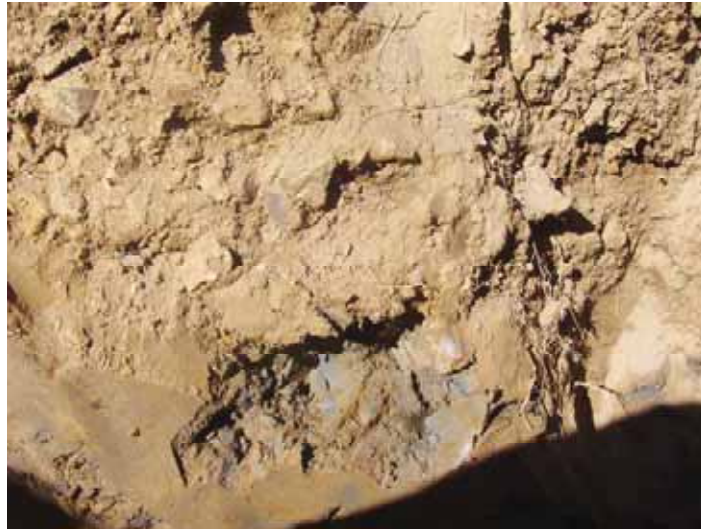
Photo 3. Trench 1, boundary between soil layers 2 (hillslope) and 3 (underlying clay)
