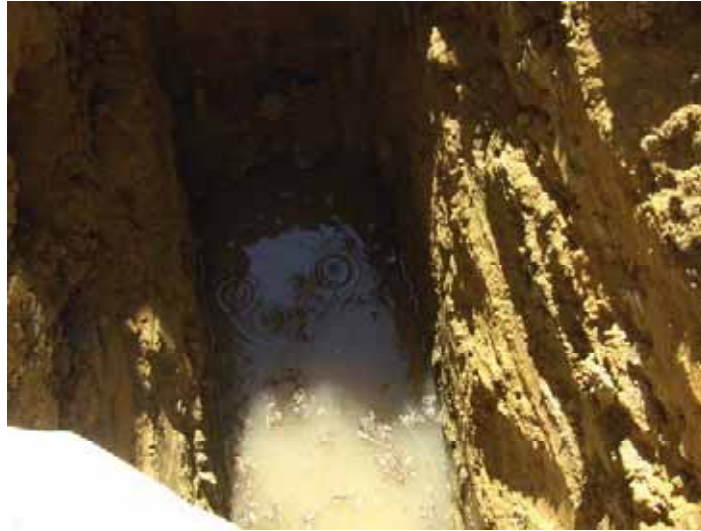
Photo 8. Trench 2, ground water. Note dark clay-dominated layer starting ~6" above water line
