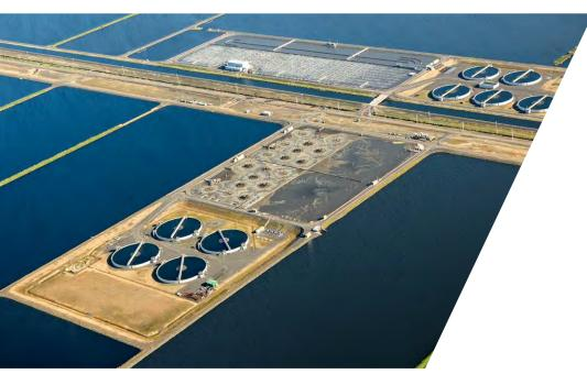
Western Treatment Plant – activated sludge plants within the treatment lagoons have enhanced nitrogen removal. Photo – Melbourne Water
